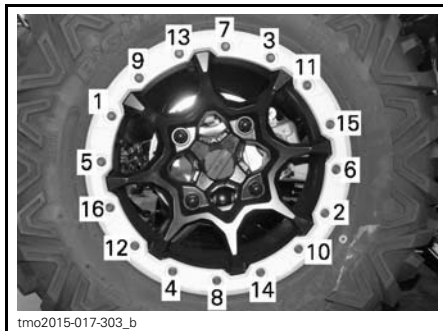
TYPICAL - TIGHTENING SEQUENCE
