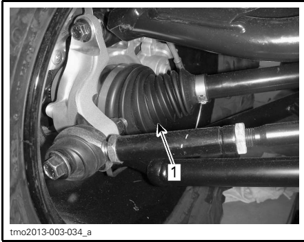
tmo2013-003-034_a REAR OF VEHICLE 1. Outer drive shaft boot
