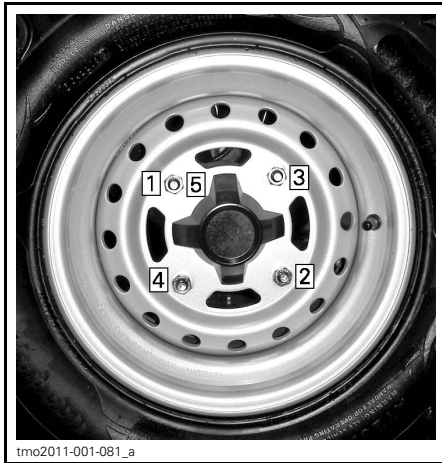
tmo2011-001-081_a TIGHTENING SEQUENCE
