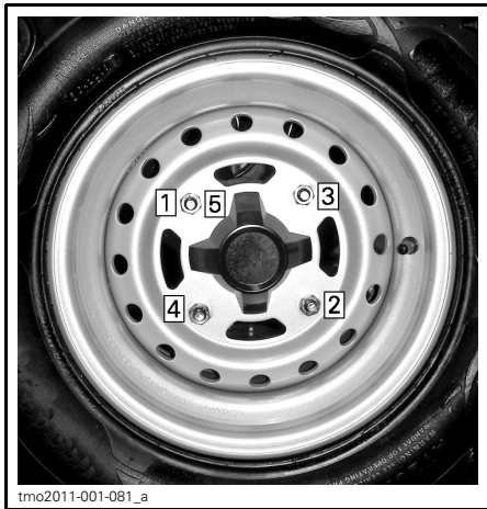
TIGHTENING SEQUENCE
