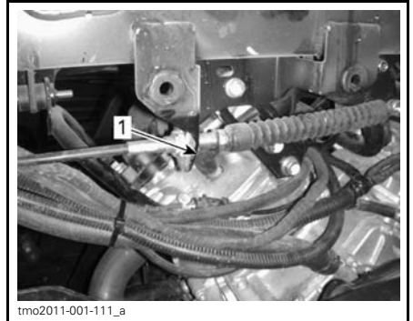
LH SIDE — FRONT CYLINDER 1. Spark plug
