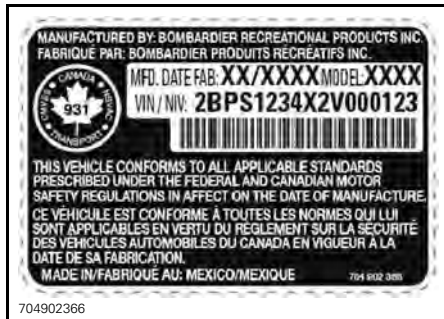
704902366 TYPICAL — VEHICLE SERIAL NUMBER LABEL UNDER GLOVE BOX
