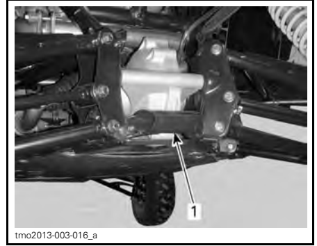
TYPICAL - REAR OF VEHICLE 1. Hydraulic jack position
