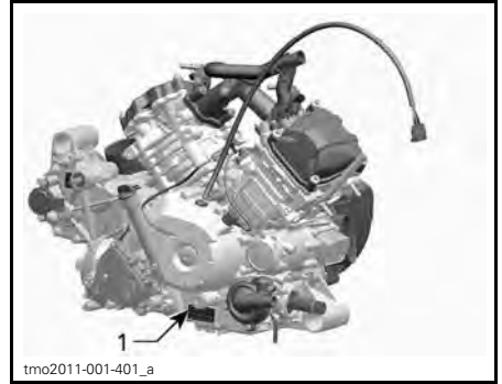
tmo2011-001-401_a TYPICAL — ENGINE SERIAL NUMBER LABEL
