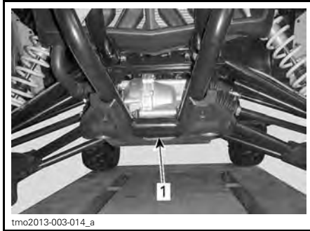
TYPICAL - FRONT OF VEHICLE 1. Hydraulic jack position
