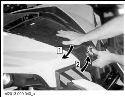
Step 1: Push down service cover and HOLD Step 2: Lift the front part of service cover
