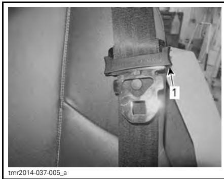
SEAT BELT ENGAGED 1. Slide locking tab
