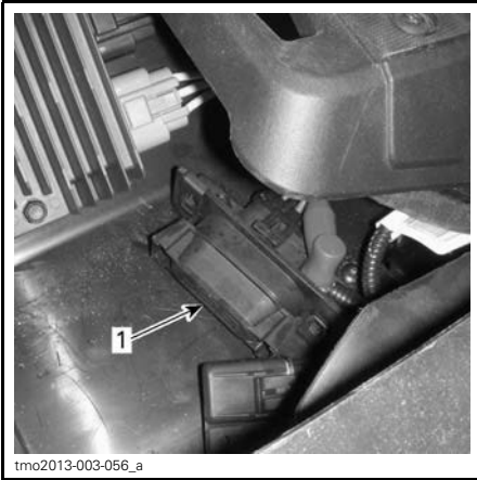
1. Auxiliary fuse box
