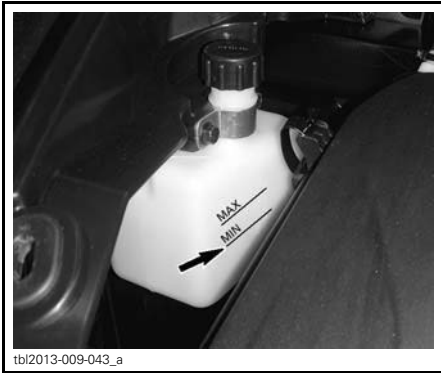
COOLANT EXPANSION TANK
