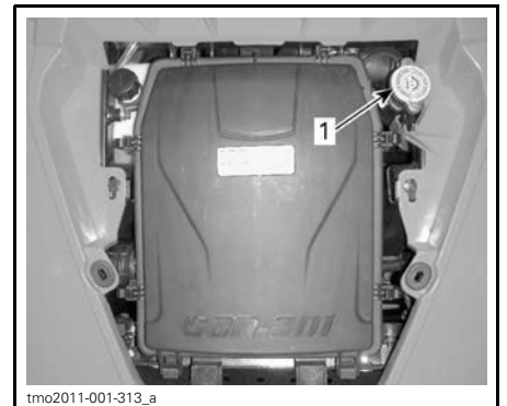
1. Radiator pressure cap
