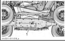
1. Cooling system drain plug access
