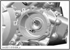
Outlet to the engine oil providing system
