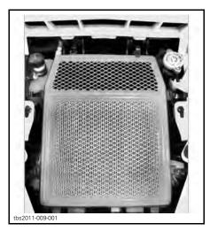
Verify that the cover fits well on the engine air filter housing before closing clamps.
