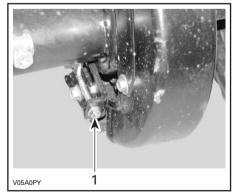
2-STROKE MODELS 1. Drive chain adjusting nut
