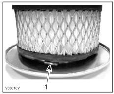
1. Gap between filter and filter base
