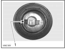
1. Interference between filter rubber edge and base bracket
