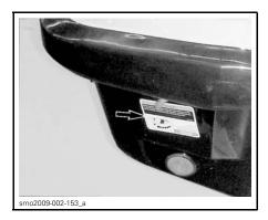
The 4-TEC<sup>™</sup> engine features a tip-over protection system (T.O.P.S.<sup>™</sup>). When the watercraft tips over, the engine is automatically stopped.
