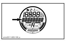
3. Press the UP button until the desired cruise speed is indicated in the numerical display.
