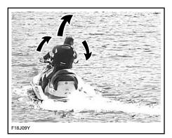
Turning the handlebar pivots the jet pump nozzle which controls the watercraft direction. Turning the handlebar to the right will turn the watercraft to the right, turning the handlebar to the left turns the watercraft to the left. The throttle should be applied to turn the watercraft.
