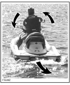
TYPICAL - STEERING DIRECTION REVERSED WHEN BACKING
