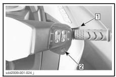
TYPICAL - ENGAGING CRUISE AT IDLE Step 1: Tap throttle to engage FORWARD Step 2: Press cruise button
