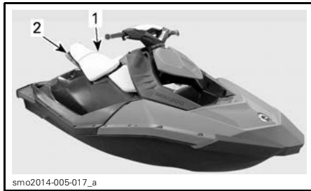
TYPICAL - PASSENGER HANDHOLDS
