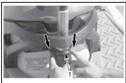
朝前推以解锁并拆下绳柱
