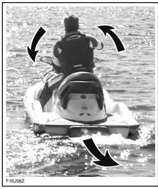
TYPICAL - STEERING DIRECTION REVERSED WHEN BACKING
