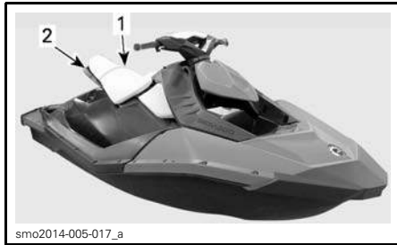
TYPICAL - PASSENGER HANDHOLDS
