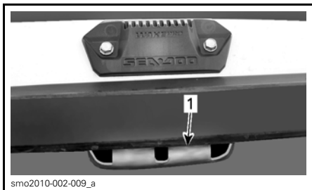
1. Hooked portion of rack in lower bracket
