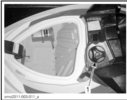
TYPICAL - FUEL TANK CAP LOCATION
