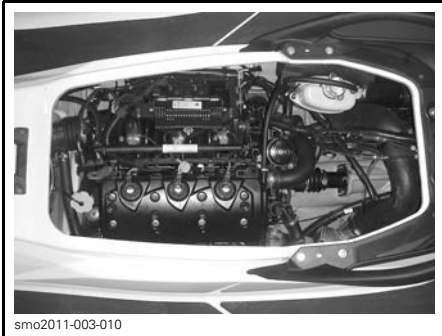
ENGINE COMPARTMENT, SEAT REMOVED
