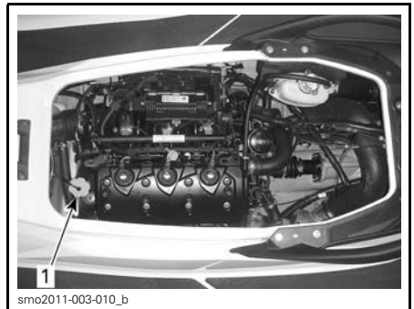
TYPICAL 1. Oil filler cap location
