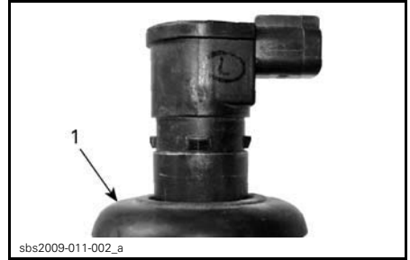
1. Rubber seal pulled down
