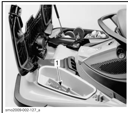
1. Fire extinguisher holder location
