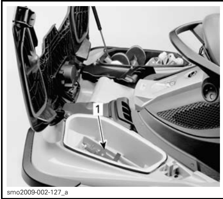
1. Fire extinguisher holder location
