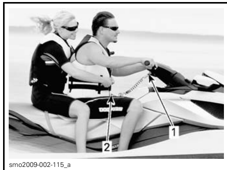
TYPICAL 1. Tether cord cap on the engine cut-off switch 2. Tether cord secured to operator's PFD
