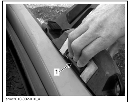
WAKEBOARD RACK REMOVAL
