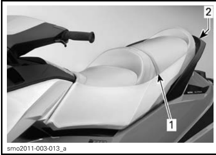
TYPICAL - PASSENGER HANDHOLDS 1. Seat strap 2. Molded grab handle
