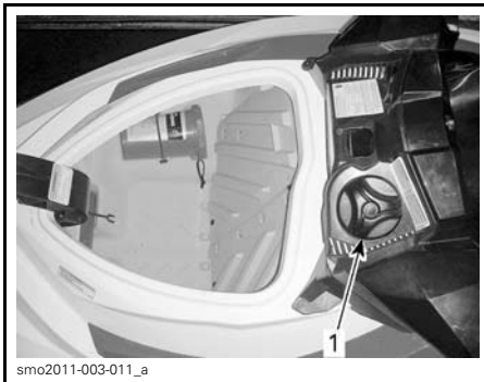
TYPICAL - FUEL TANK CAP LOCATION
