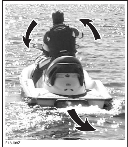
TYPICAL - STEERING DIRECTION REVERSED WHEN BACKING
