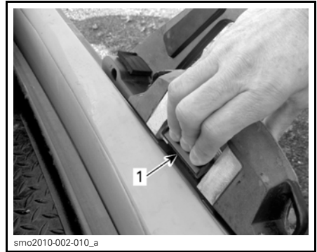
WAKEBOARD RACK REMOVAL
