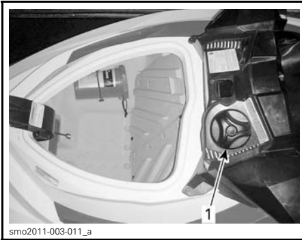
TYPICAL - FUEL TANK CAP LOCATION
