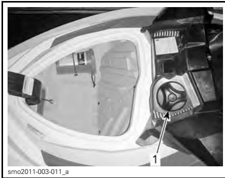
TYPICAL - FUEL TANK CAP LOCATION
