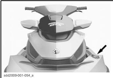
TYPICAL - FUEL TANK CAP
