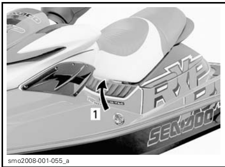
TYPICAL 1. Air intake opening
