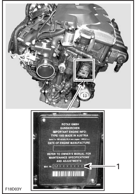
TYPICAL 1. Engine Identification Number (E.I.N.)
