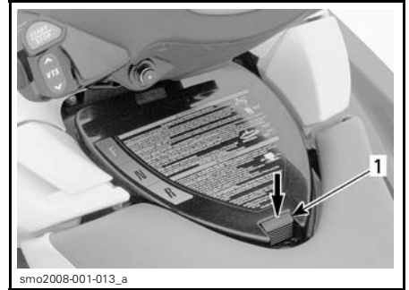
RXP MODELS — PUSH ON LATCH TO RELEASE 1. Cover latch
