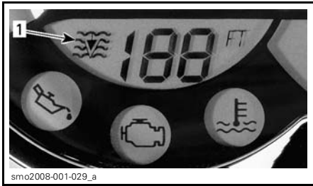
TYPICAL — UNDER RPM 1. Water depth
