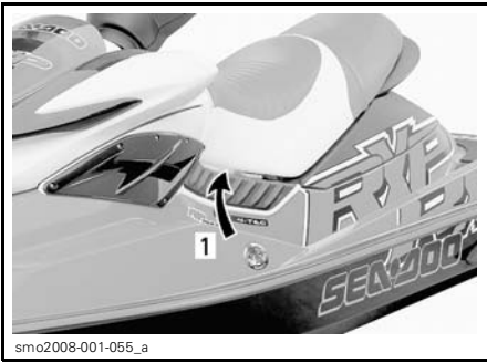
TYPICAL 1. Air intake opening
