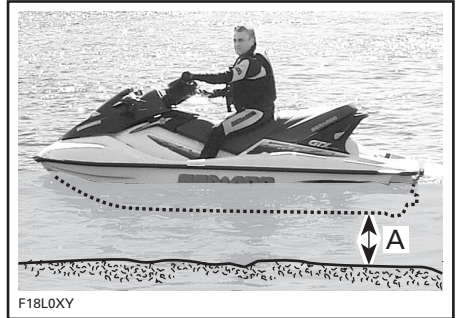
A. Maintain at least 90 cm (3 ft) underneath the lowest rear portion of the hull when all passengers are aboard
