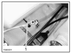
**TYPICAL** Hose pincher installed on engine drain hose
