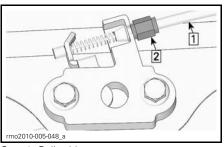
Step 1: Pull cable Step 2: Turn adjuster
