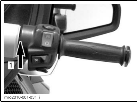
CRUISE CONTROL PREVIOUSLY SET 1. Push up button to increase the speed setting
