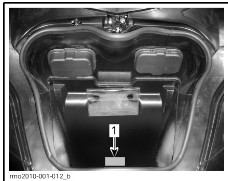
1. Label 3 located in the front storage compartment
