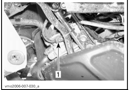
LH SIDE — FRONT CYLINDER 1. Spark plug
