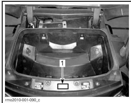
1. Label 5 located in the top storage compartment
