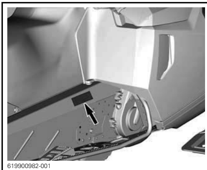
TYPICAL - NRMM IDENTIFICATION ON RH SIDE OF TUNNEL
