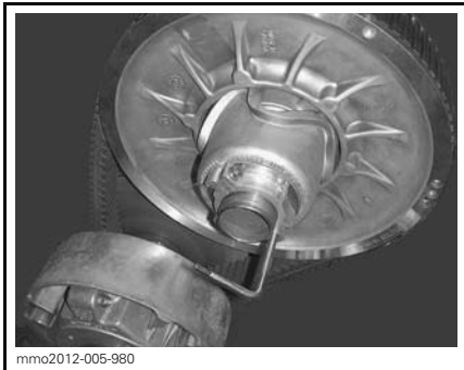
PULLEY EXPANDER INSTALLED ON ADJUSTER HUB
