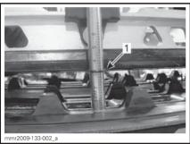
9. Read load recorded by the upper O-ring on the tensiometer.
