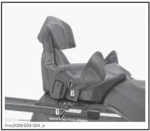
Step 1: Pull rubber tab Step 2: Lift RH side
