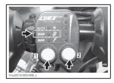
To adjust spring preload push the left button till the MAN/spring figure led lights up. Push the right knob to set the preload. Upwards is more preload and down is less preload.
