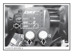
To increase or decrease the damping push the left knob till the MAN/shock figure led lights up. Push the right knob to set the damping. Upwards is more damping and down is less damping.
