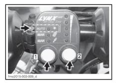
To use preselected values push the left button till AUTO led lights up. Push the right knob to set the preselected spring preload and damping force. Upwards is more spring preload/damping force and down is less spring preload/damping force.
