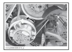
Pull the rope using a sharp, crisp pull so the rope comes free of the drive pulley.
