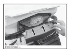
2. Pass the retaining straps behind the taillight.
