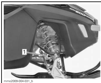
TYPICAL - CAM TYPE PRELOAD 1. Adjustment cam
