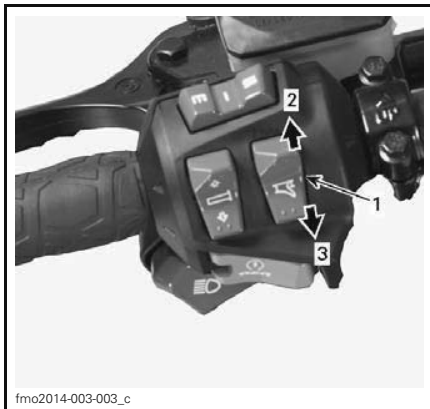
TYPICAL 1. Heated throttle lever switch 2. Increase heat (Warmer) 3. Decrease heat (Colder)
