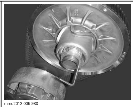
PULLEY EXPANDER INSTALLED ON ADJUSTER HUB
