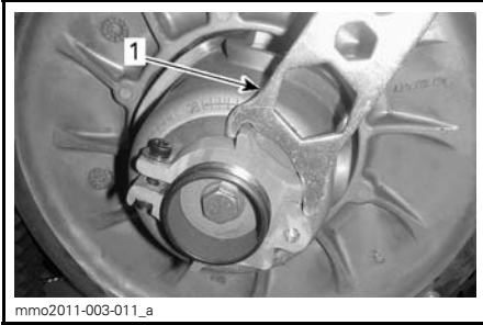
ALUMINUM ADJUSTER HUB 1. Suspension adjustment tool
