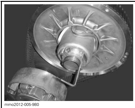
PULLEY EXPANDER INSTALLED ON ADJUSTER HUB
