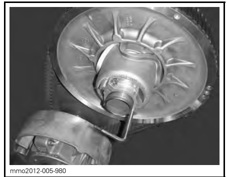
PULLEY EXPANDER INSTALLED ON ADJUSTER HUB
