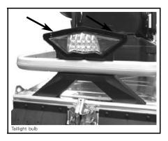
Led taillight leds cannot be replaced. If failed change taillight assy. Fasten new taillight by screws.
