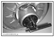
5. Open the driven pulley by screwing the tool in
