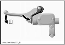
TYPICAL — RELEASE MECHANISM Step 1: Squeeze brake lever
