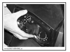
Unplug burnt bulb connector. Remove the rubber boot.
