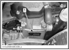
**1200 4-TEC ENGINE** Engine serial number
