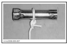
Attach the other end of emergency rope to the starter clip supplied in the tool kit.
