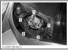
Step 1: Push both sides Step 2: Pull to release
