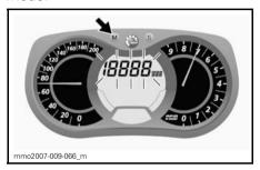
Push and hold the SET (S) button within 5 seconds to reset.
