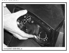
Unplug burnt bulb connector. Remove the rubber boot.
