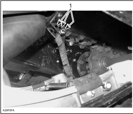
1. Bolt stopper strap to a different hole
