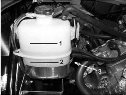
YETI V-800-EXPANSION TANK NEAR THE MUFFLER
