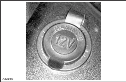
TYPICAL — ELECTRIC POWER OUTLET
