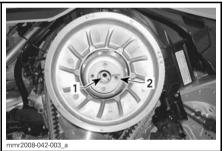
DRIVEN PULLEY 1. Locking nut 2. Adjustment ring
