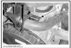
600 HO E-TEC<sup>®</sup> ENGINE — RH SIDE OF ENGINE COMPARTMENT 1. Engine serial number
