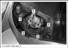
Step 1: Push both sides Step 2: Pull to release 1. Spindle
