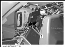
RH SIDE OF ENGINE COMPARTMENT 1. Fuse location
