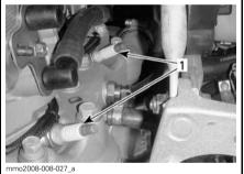
LH SIDE OF ENGINE COMPARTMENT 1. Spark plugs
