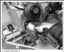
593SS ENGINE 1. Engine serial number
