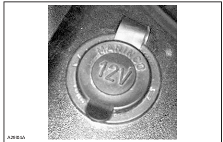
TYPICAL — ELECTRIC POWER OUTLET
