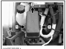
FUSE BOX COVER Step 1: Push on tabs Step 2: Pull cover
