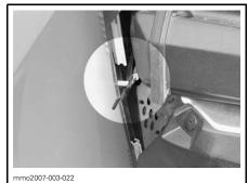
FRONT RETAINING PIN PROPERLY SECURED
