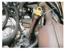
4. Open drainplug (1) and drain oil into the oil waste can.
