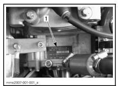
LIQUID-COOLED — V-810 ENGINE TYPE 1. Engine serial number
