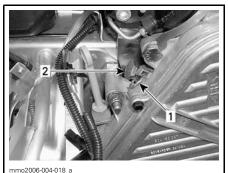
TYPICAL — RH SIDE OF ENGINE COMPARTMENT 1. Hair pin 2. Adjustment screw
