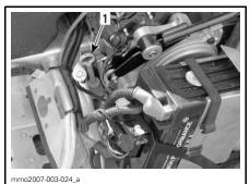
TYPICAL — RH SIDE OF ENGINE COMPARTMENT 1. Dipstick location
