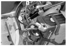
2) Open the drainplug (1) and let oil run out from chaincase into a oil waste can.
