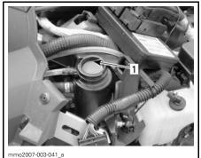
COOLANT TANK — LH SIDE 1. Fill to maximum line if necessary
