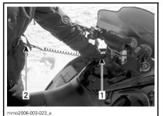
**TYPICAL** 1. Snap over post 2. Attach to eyelet
