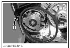
Step 1: Place belt between drive pulley sheaves
