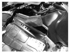
Check that the air silencer is clean and dry and properly reinstall the filter.
