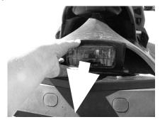
Turn bulb base to the counter clockwise to open the bulb base from tail light.
