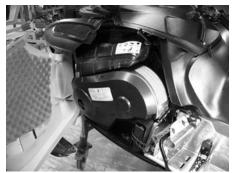
Lift up the intake silencer clamp.
