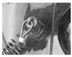
It shuts off engine preventing snowmobile to runaway if the operator falls off the vehicle accidently.
