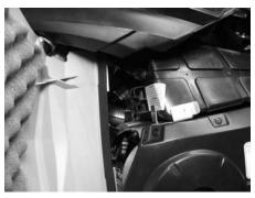
Some models: To keep spare spark plugs dry and prevent shocks that might affect the adjustment or break them, a holder is provided in engine compartment.
