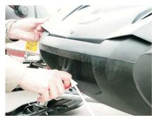
Open electrical connector at right side of vehicle by pressing the connector locking before lift up upper hood.
