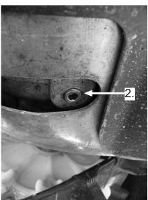
When oil is out from chaincase, close the drainplug.
