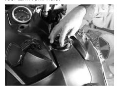
Lift console front edge up (pin in the rubber ring).
