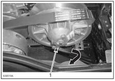
1. Tighten to open pulley
