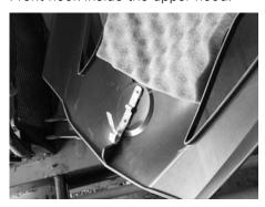
Opening for the hook when installing upper hood.
