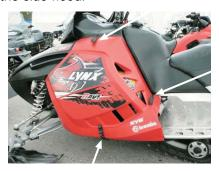
If you like to remove complete side panel, open the lockings and remove side hood.
