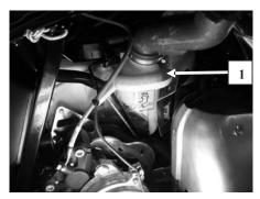
1. Max oil level. (Do not overfill)
