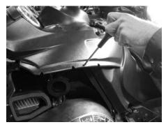
Open console big plastic nut round the fuel tank refill hole.
