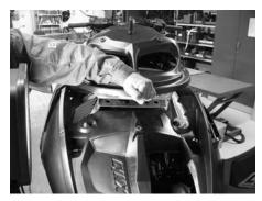
Lift the console rear edge until you have enough space to work with head lamp bulbs.
