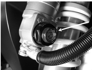
Too hard of adjustment 1. Steering hard to turn - Decrease spring preload
