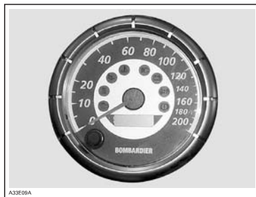
Push and hold the button for 2 seconds to reset the hourmeter.
