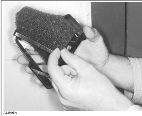
Removal of filter from its grill
