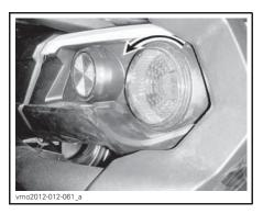
Disconnect the light bulb connector.
