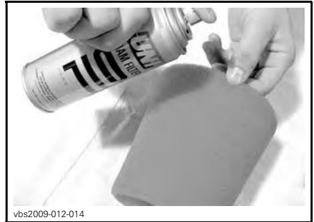
TYPICAL - OIL THE FOAM FILTER
