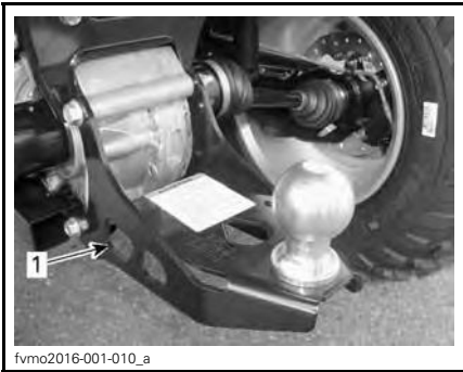
TYPICAL - REAR TIE-DOWN POINT LOCATION
