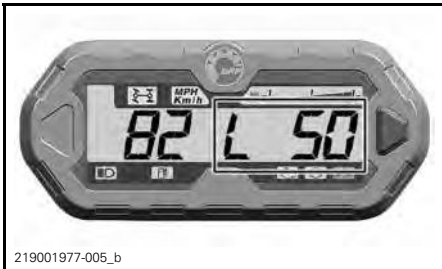
L AND SPEED LIMIT FLASHING
