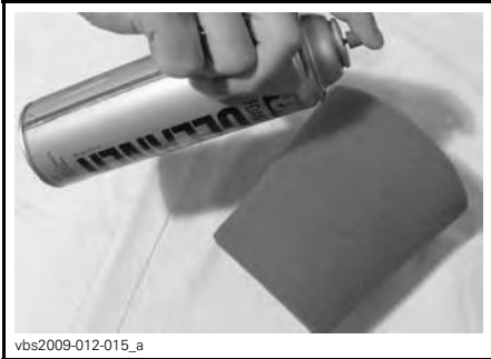
TYPICAL - SPRAY THE FOAM FILTER
