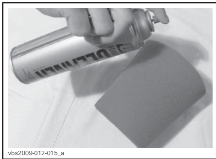
TYPICAL - SPRAY THE FOAM FILTER
