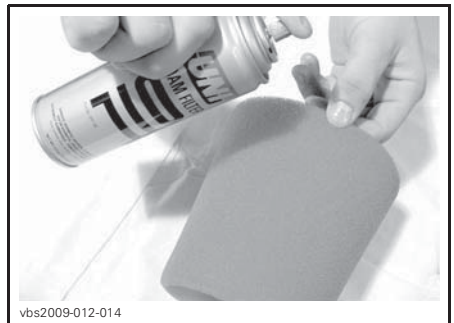
TYPICAL - OIL THE FOAM FILTER
